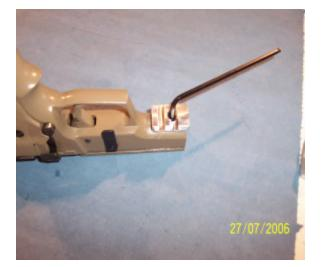
Next, you must grind/file down the screw on the inside of the dust cove. This is where the recoil spring moves back and forth, if you do not grind/file the screw down, it will jam the slide.
