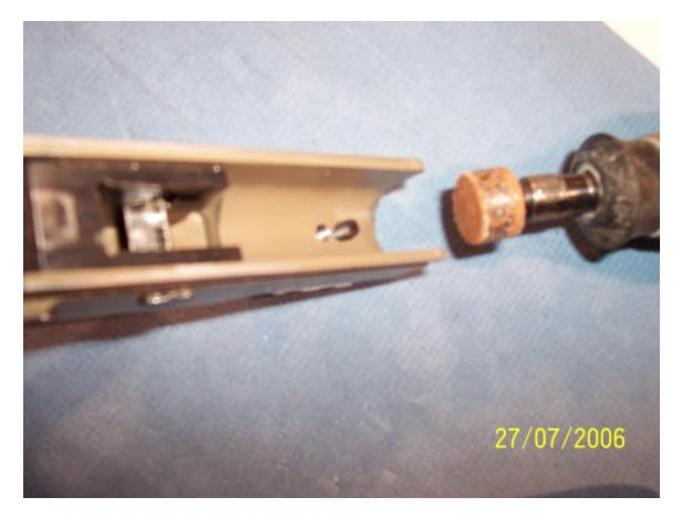
Next, remove Tactical Rail and finish using desired method. Then reassemble Tactical Rail using a tread locking liquid.
