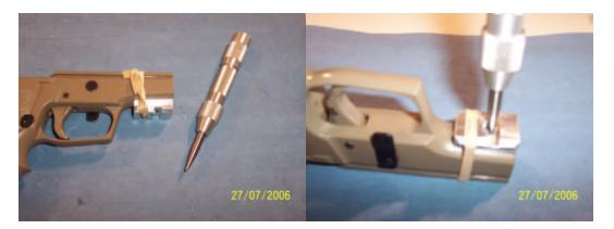
Next, drill the hole. Use a #29 drill (.136) For this frame we did use the elastic and a cordless hand drill. Cordless drill, good. Drill press or mill best
